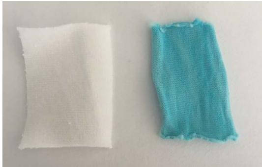
**Figure 3.** Cotton fabric (left) and CuBTC deposited cotton fabric (right).
