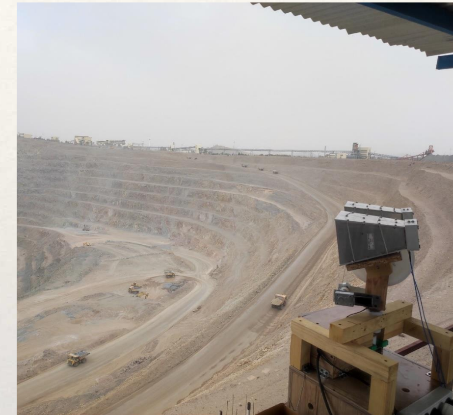
Radar System for Mining Wall Monitoring
